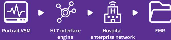
Connectivity to Cerner<sup>™</sup> Millennium<sup>™</sup> EMR via CareAware<sup>™</sup> VitalsLink<sup>™</sup> with help of an iBus<sup>™</sup> protocol
