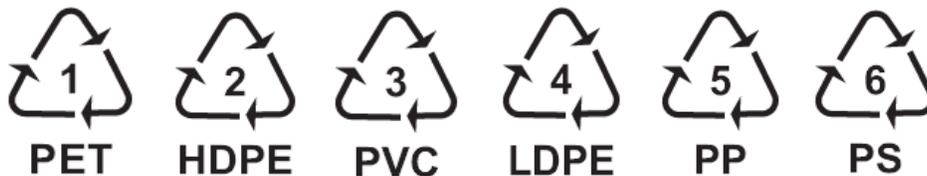
Material markings according to the Industry Standards ISO 1043 and ISO 11469 may be used if it is confirmed that they will comply with the standard GB 18455-2001. Examples of the ISO codes include:
