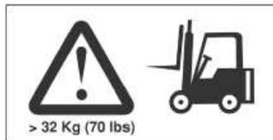
Weight restriction – For units over 32 kg (70 lbs.), design packaging to be handled by mechanical handling equipment (hand truck, cart, fork lift or hoist)
